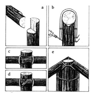
a) Post and rail halved, then roped. b) Rail notched into top of post, secured with rope, or wire, then stapled to post. c) Rails halved, and d) cut diagonally, then butted together. e) roping a corner.
