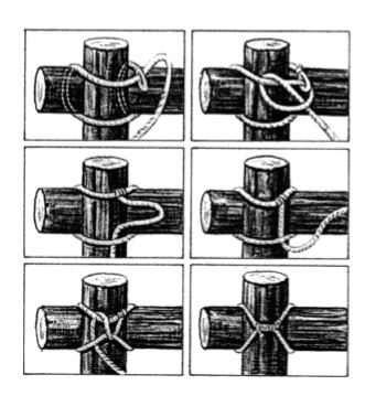
Roping rails to posts is safer than using nails, bolts, or wire. Polypropylene 1/4in (6mm) diameter rope does not break, is easy to handle, and can be cut in an emergency. After roping, trim the posts.
