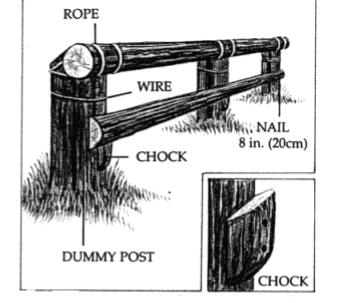
Strong, inviting post and rails: the top rail is roped to the main post and supported on an adjustable "dummy" post. The lower rail, slightly prominent, rests on a chock at one end, for quick release.
